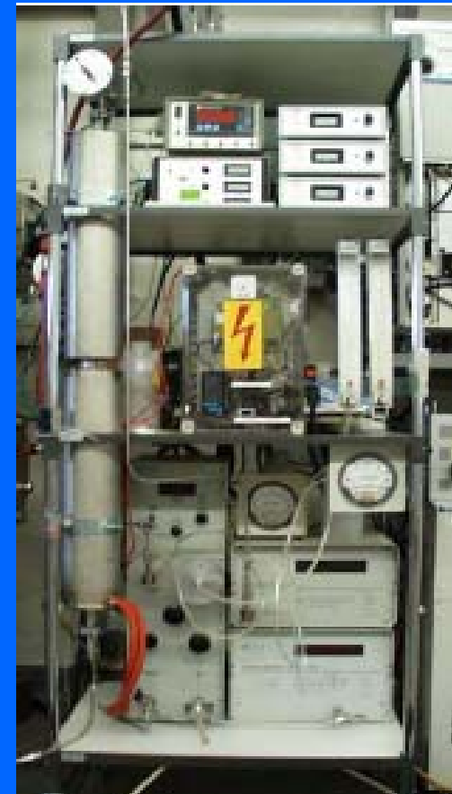
EMPA measuring equipment (on top: control unit, middle: heating unit for thermobalancer (TD) and flow control, bottom: Differential Particle Analyzer (DMA) and 2 Condensation Particle Counters (CPC))
