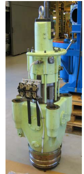
Liquid cooled exhaust valve spindle
