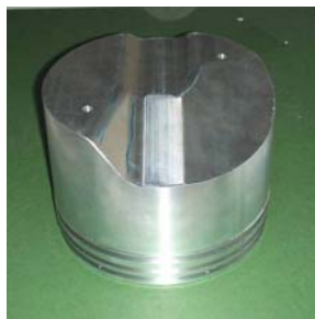
Extended piston for optical setup
