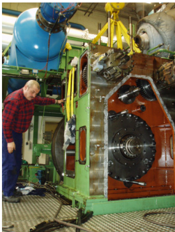
Building up of the test engine with new components and mounting on the test bed.
