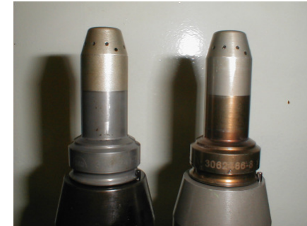
Compound fuel valve nozzle
