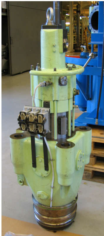
Liquid cooled exhaust valve spindle
