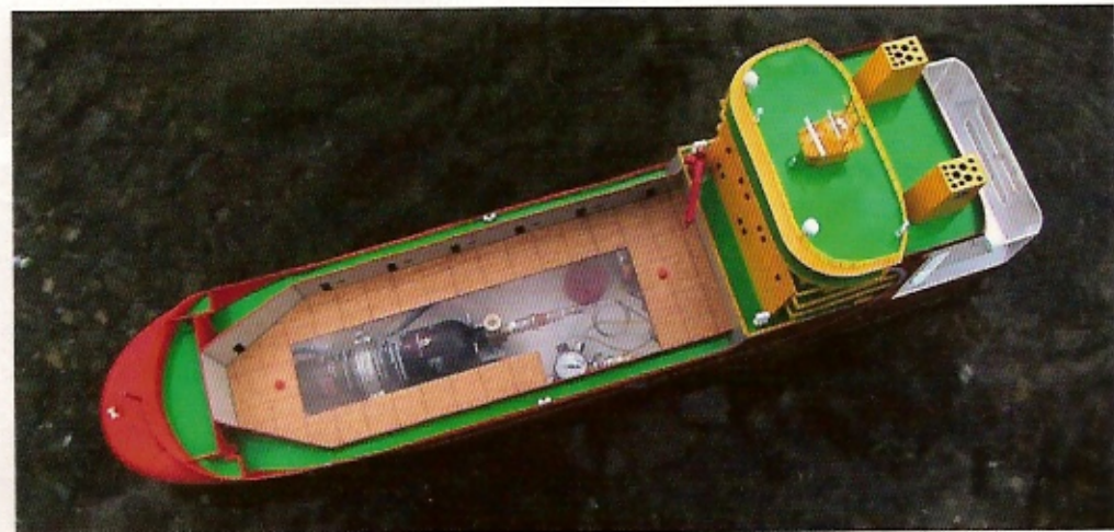
■ The FellowSHIP scale model (1:84) of the offshore supply vessel is operated remotely and powered by hydrogen and proton exchange membrane (PEM) fuel cells
