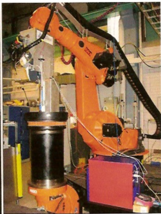
■ A piston ring friction tester (left) and a cylinder liner for a 'hot'-operating engine (right) have both been developed as part of the Hercules project
