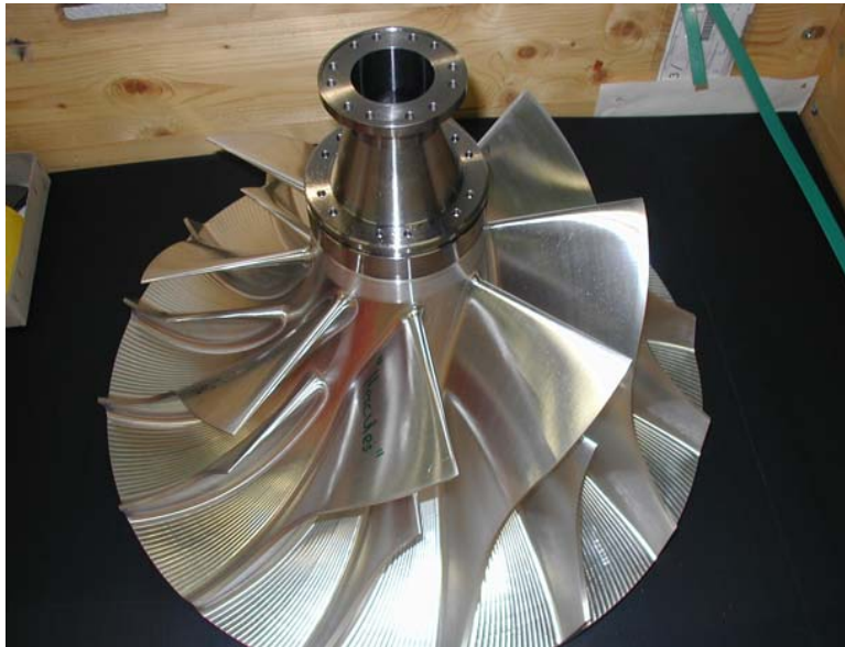
PTI: compressor wheel with coupling parts
