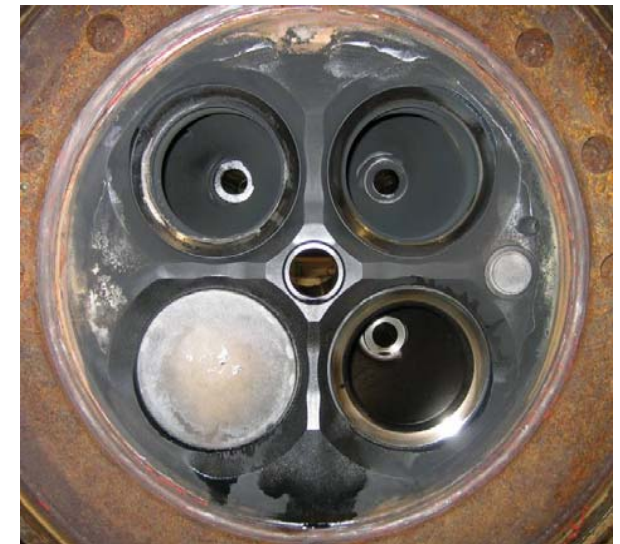
Prototype seat rings assembled in cylinder head
