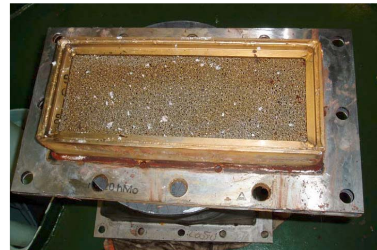
Metal Foam Water Mist Catcher with deposits
