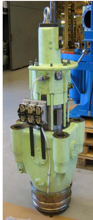
Liquid cooled exhaust valve spindle
