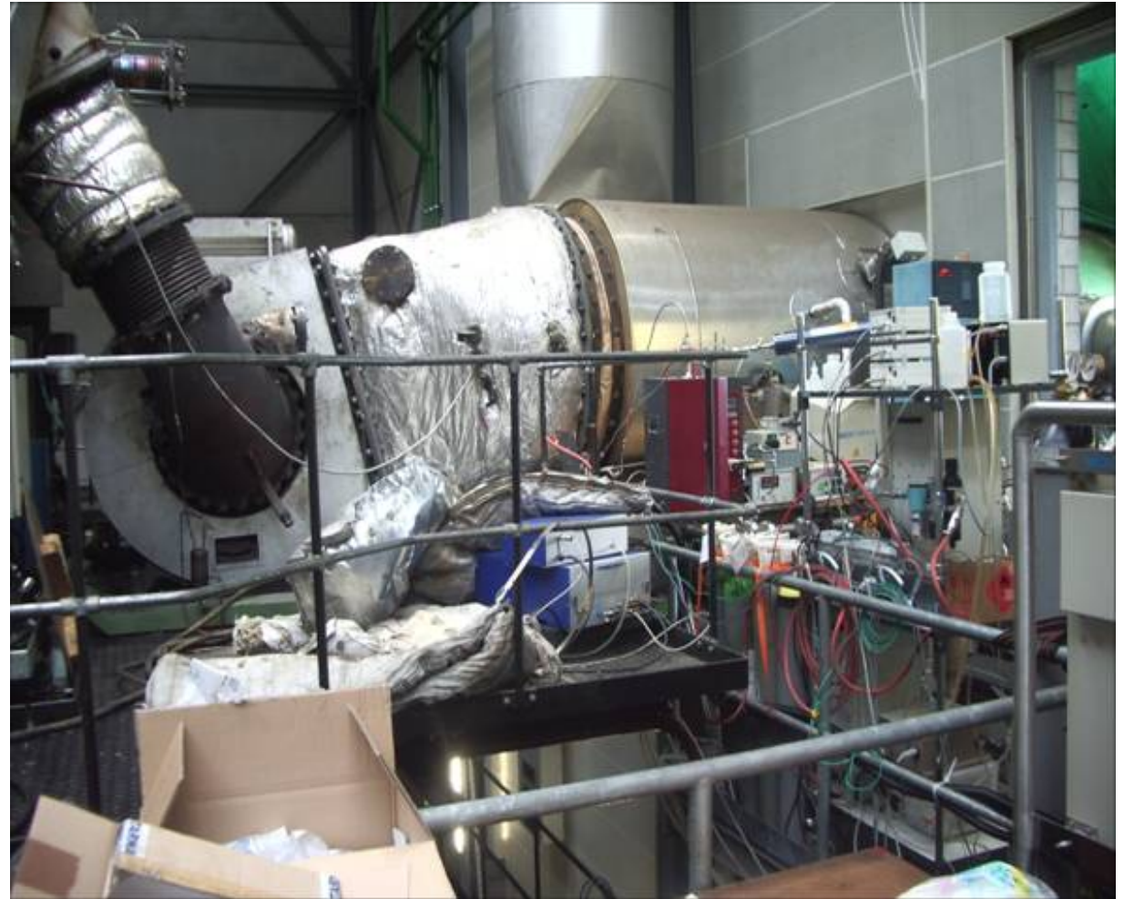
Experimental emission measuring equipment and general setup on test engine
