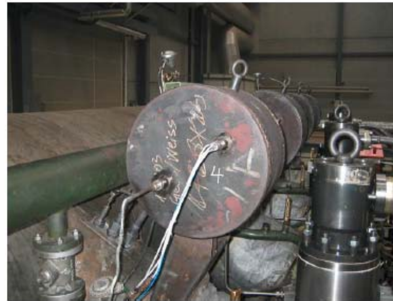
Pictures of manufactured and installed bypass receivers on the RTX-3 test bed engine
