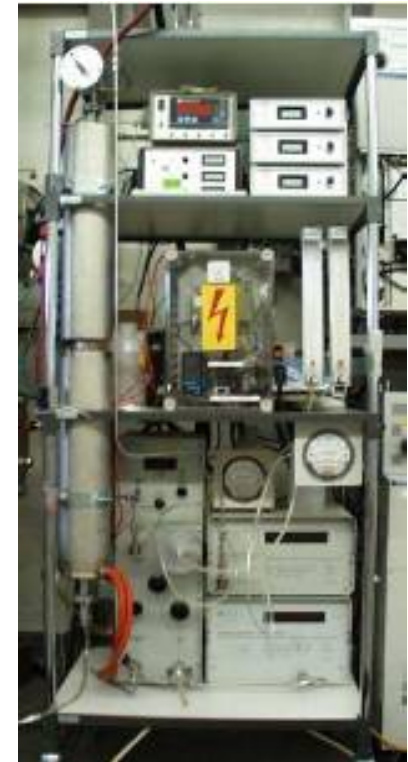
EMPA measuring equipment (on top: control unit, middle: heating unit for thermomixer (TD) and flow control, bottom: Differential Particle Analyzer (DMA) and 2 Condensation Particle Counters (CPC))
