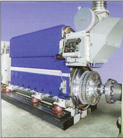
Testbed engine used in task 11.2 investigations into intelligent engine control.
